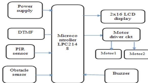
Figure 6: Block diagram of detection robot [10]
