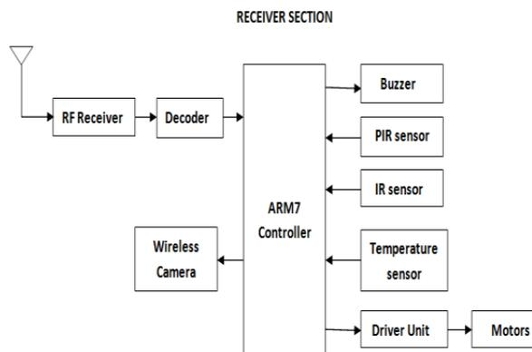
Figure 3: RF receiver and Decoder [7]
